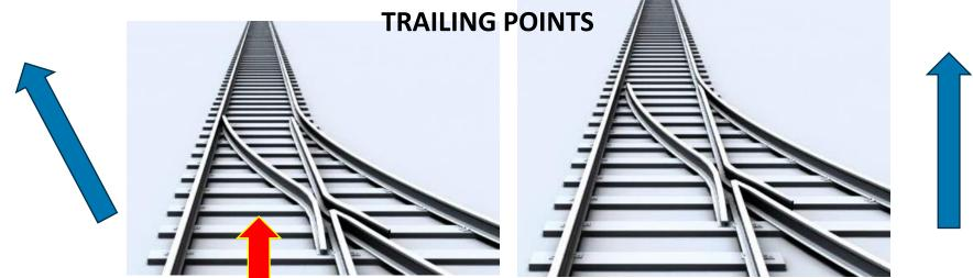
Both of the points in the images above are defined as Trailing, because you cannot see the ends of the point toes, and you would move over the crossing section of the points before the Switch rail section. If you look carefully at the switch rails in these two images you can see that the route setting is different in both of the images.
