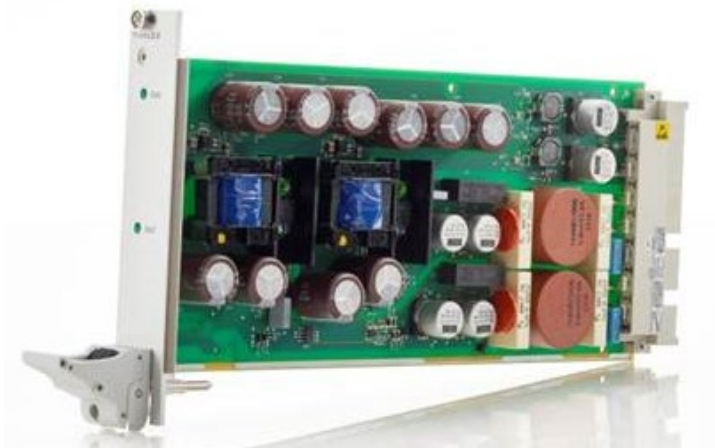
Figure 11 - Internal Supply Board
