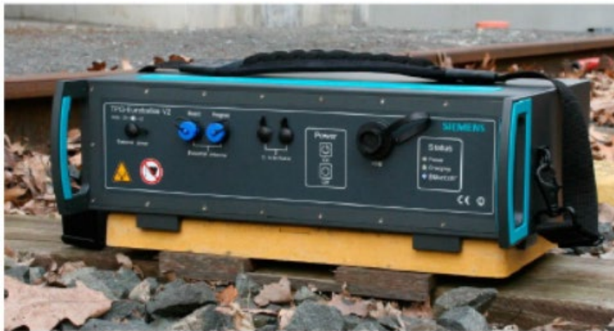
Figure 4 - TPG Base Unit Positioned on Eurobalise.
