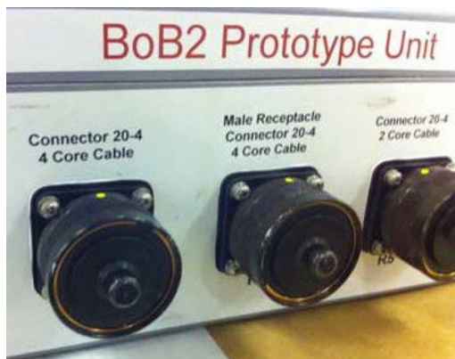
Figure 4 – Break Out Box with environmental covers in place
