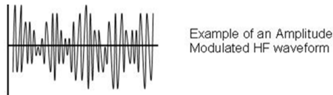
Figure 6 – Amplitude Modulated HF waveform
