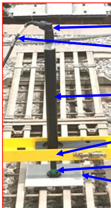
Figure 1: Measuring TPWS Field Strength - Commissioning Test
