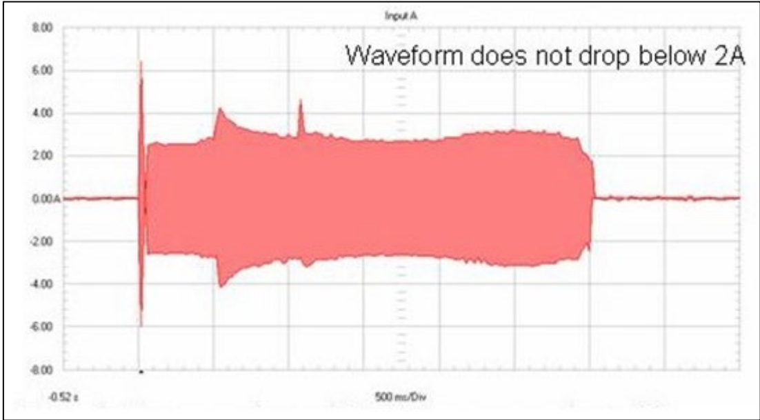
Figure 1 – Trace 1: Current probe on L2, running current above 2A Dummy load resistors not necessary
