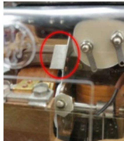
Figure 4 – Vane in the Energised position
