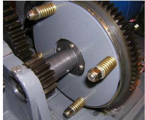
Figure 24 - Mechanical clutch on a HW1000 machine
