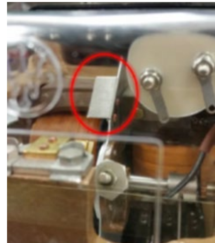
Figure 1 – Vane in the Energised position
