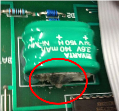
Fig 6 – Close up of a corroded battery terminal
