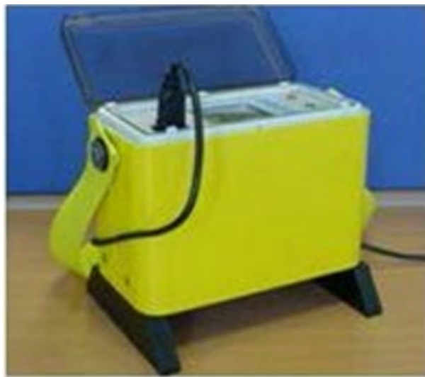
Figure 3 - IPM Systems Trackside Magnet Tester
