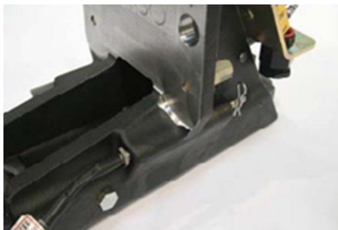
Figure 14 – Pencil heater fitted into lock body
