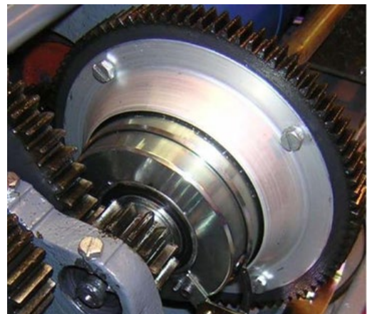
Figure 25 - Electromagnet clutch on a HW2000 machine
