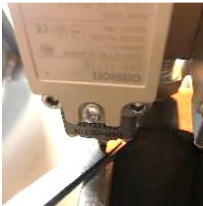
Figure 6 - 1.5 mm gauge (Inserted)
