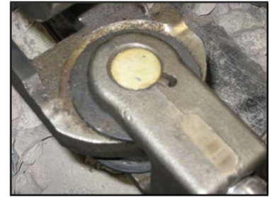
Figure 7 - Drive Lock Slide / Drive Bracket Coupling
