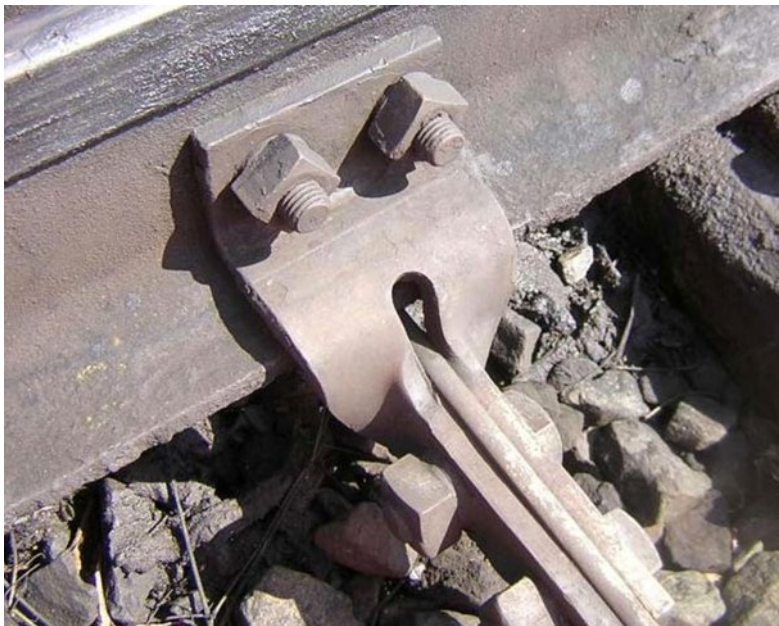
Figure 8 – Black stretcher bar bracket with square nut fastenings
