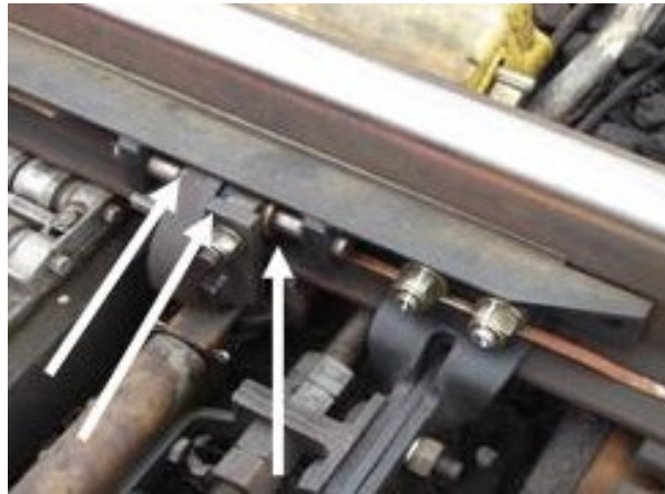
Figure 1 - Mk 2 pivot pin lubrication points
