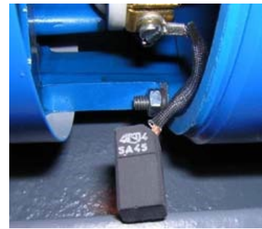
Figure 9 - A new motor brush before insertion in its holder
