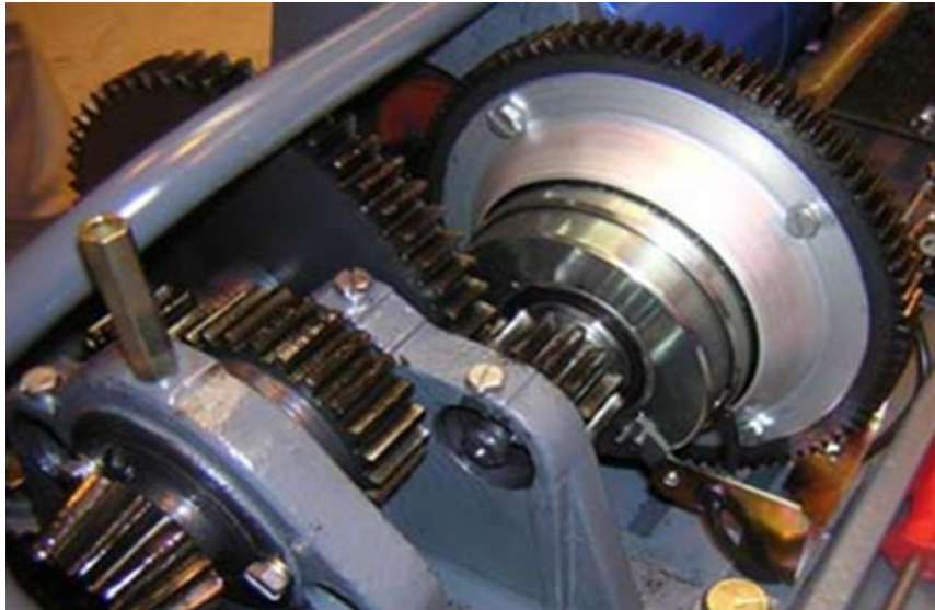
Figure 7 - Gear train on a HW2000 machine with the gearbox cover removed
