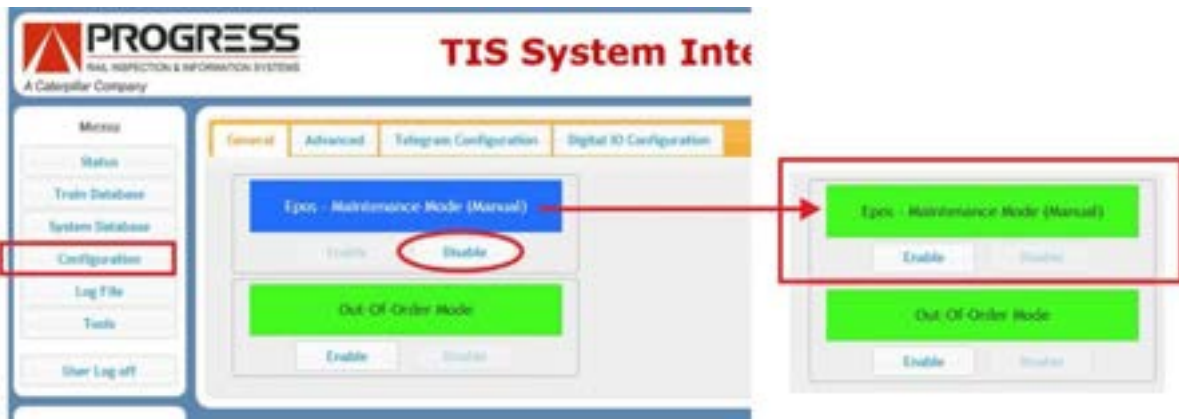
Figure 11 - Maintenance mode in FUES-EPOS GUI
