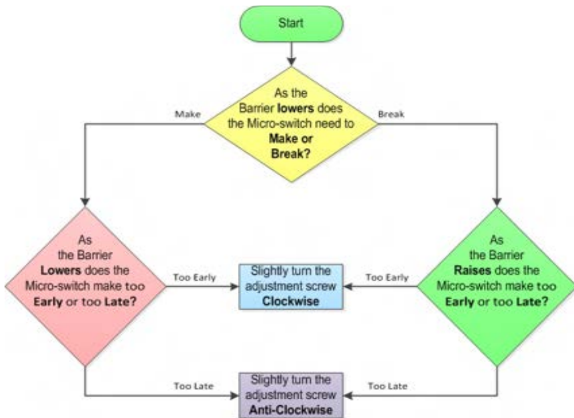
Flowchart 1 – Micro-switch adjustment process
