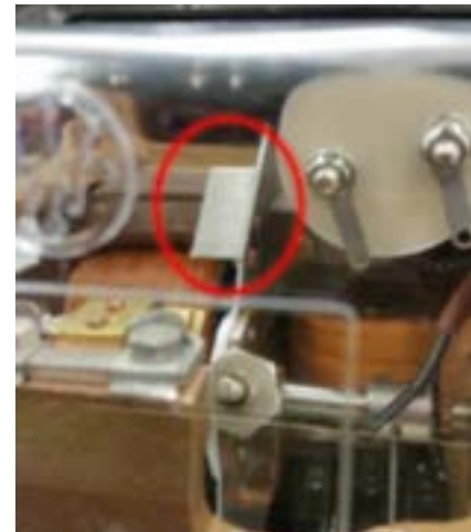
Figure 1 – Vane in the Energised position
