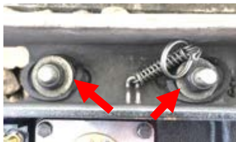
Figure 3 - Examples of Damaged, Worn and Perished Vibro Washers
