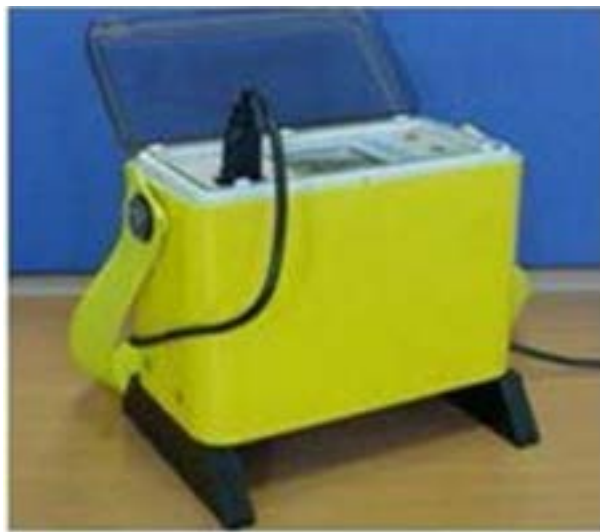
Figure 3 - IPM Systems Trackside Magnet Tester
