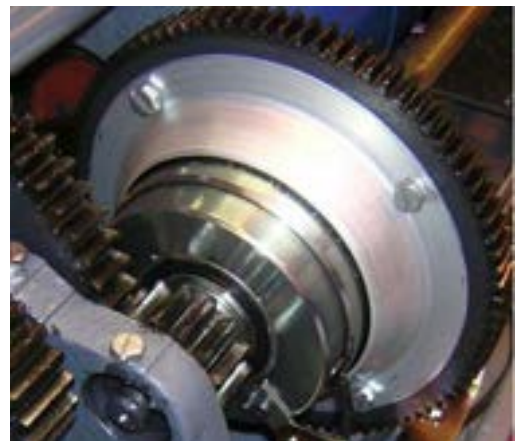
Figure 25 - Electromagnet clutch on a HW2000 machine
