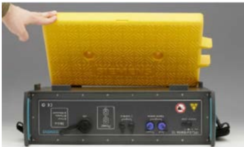
Figure 5 - Eurobalise Positioned on TPG Base Unit
