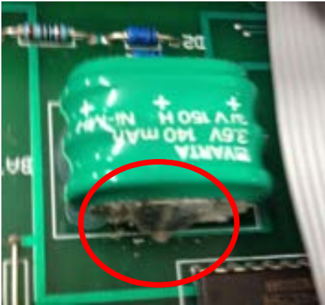
Fig 6 – Close up of a corroded battery terminal
