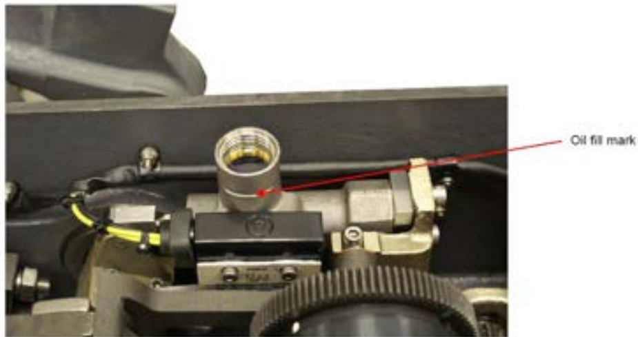
Figure 1 – Dashpot Oil Fill Mark
