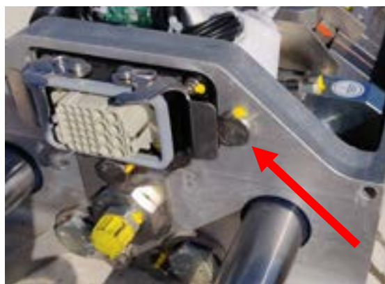
Figure 6 - Protective vent indicated by arrow one on each side of the DLD
