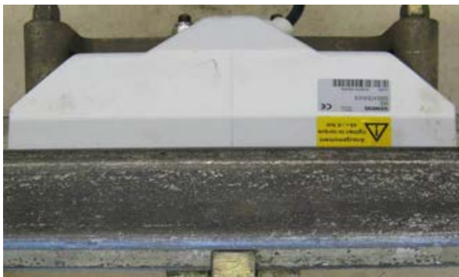
Figure 2 – Too close to the rail
