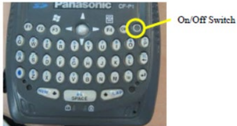
Figure 9 – Location of On/Off Switch
