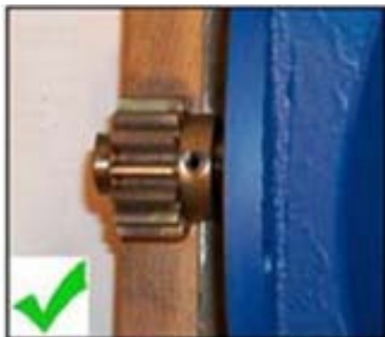
Figure 5 – Correct spirol pin position
