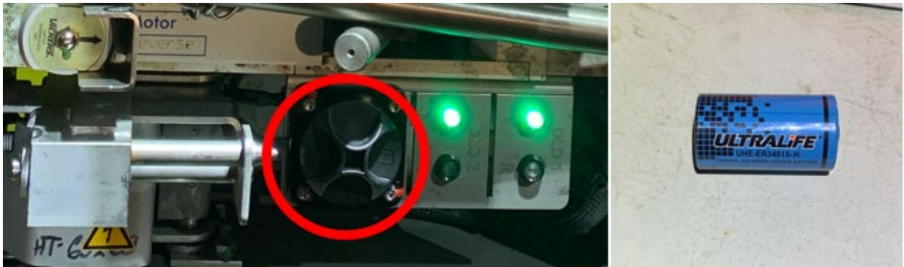
Figure 2 - Location of local indication battery within Unistar HR power pack
