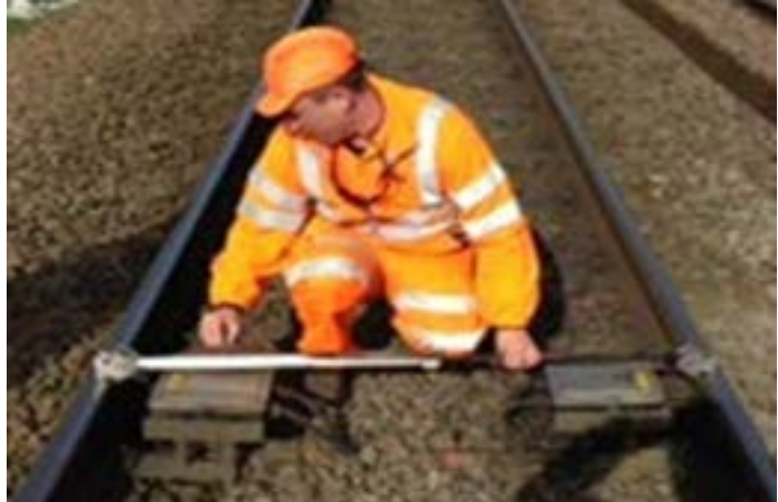
Figure 3 – Using the Gauge
