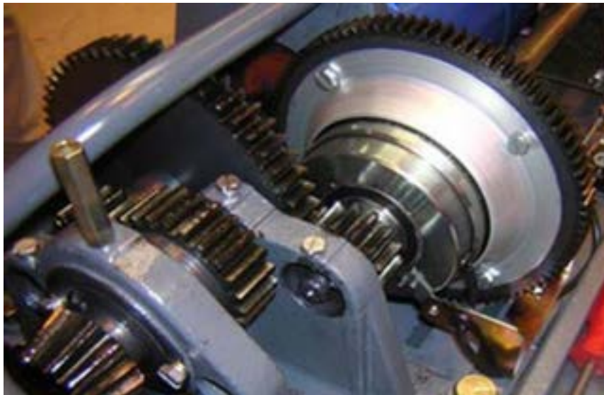
Figure 7 - Gear train on a HW2000 machine with the gearbox cover removed
