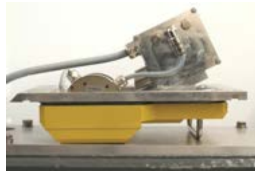
Figure 9 - HWD EPOS-Unit placed on the sleeper
