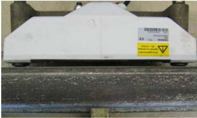
Figure 3 – Too far away from the rail
