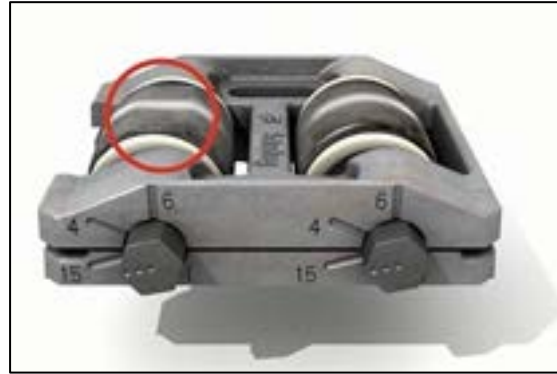
Figure 3 – Check for movement and flat spots
