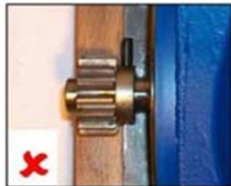
Figure 6 – Spirol pin working loose
