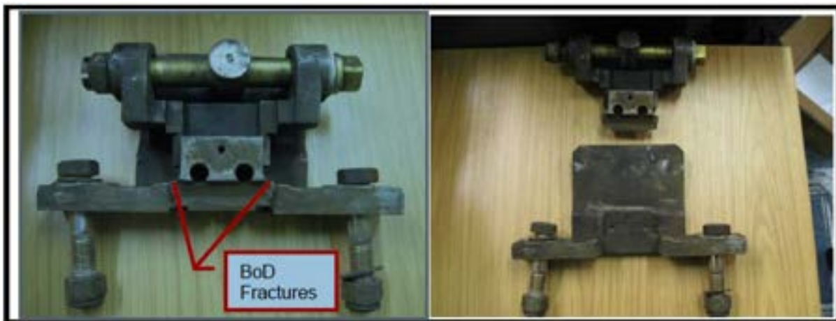
Figure 1 – Mk1 Break Out Device (BOD) fractures Checking BOD’s for Operation
