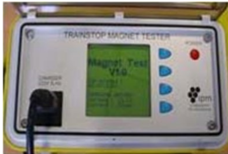
Figure 6 - Display showing information page (battery being charged)
