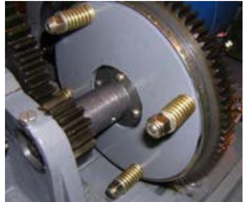
Figure 24 - Mechanical clutch on a HW1000 machine
