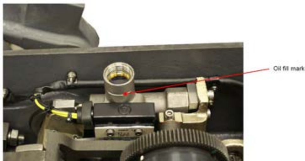
Figure 2 – Dashpot Oil Fill Mark
