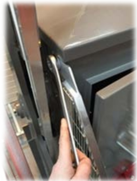
Figure 15 – Top M20 Fixings
