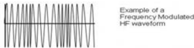
Figure 7 – Frequency modulated HF waveform
