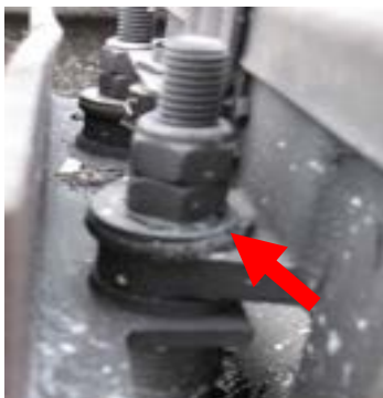
Figure 3 - Examples of Damaged, Worn and Perished Vibro Washers
