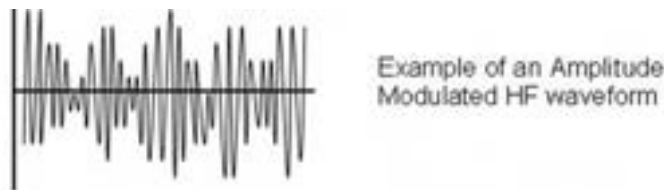
Figure 6 – Amplitude Modulated HF waveform
