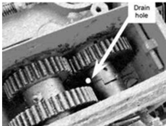
Figure 4 - Location of drain hole in gear wheel compartment
