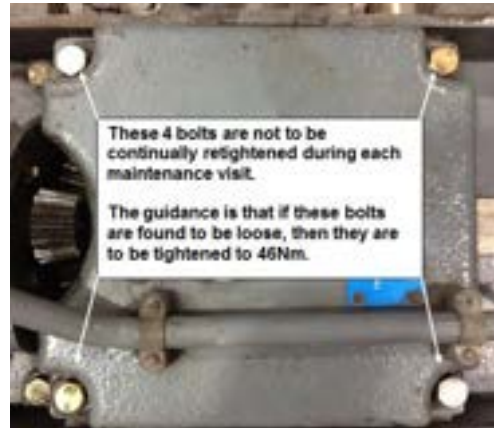
Figure 13 – Mounting plate bolts
