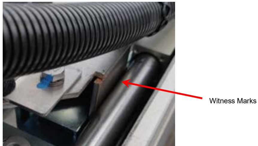
Figure 1 - Detector Plate witness marks indicating optimal set up between marks for 0mm and 2.5mm
