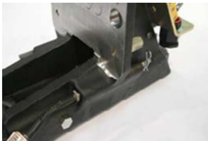
Figure 14 – Pencil heater fitted into lock body
