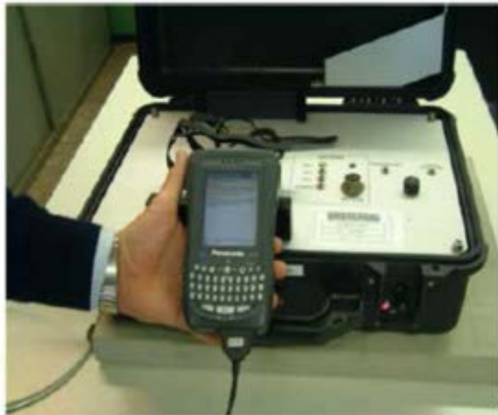
Figure 17 – Checking the Air Gap
