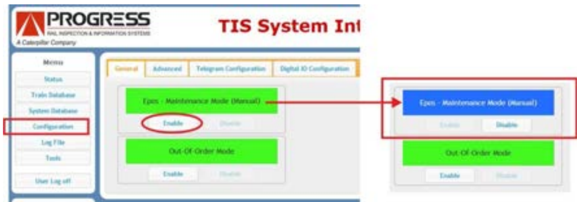
Figure 4 - Maintenance mode in FUES-EPOS GUI
