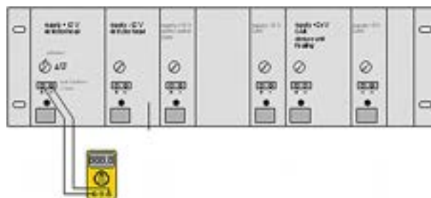
Figure 10 - Method for taking voltage readings on the power supply modules.
