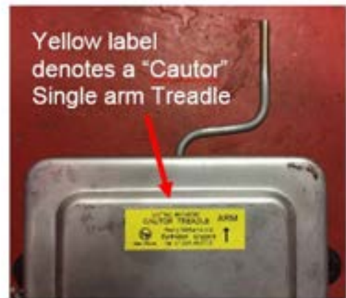
Figure 3 - An example of the direction indicating arrow
