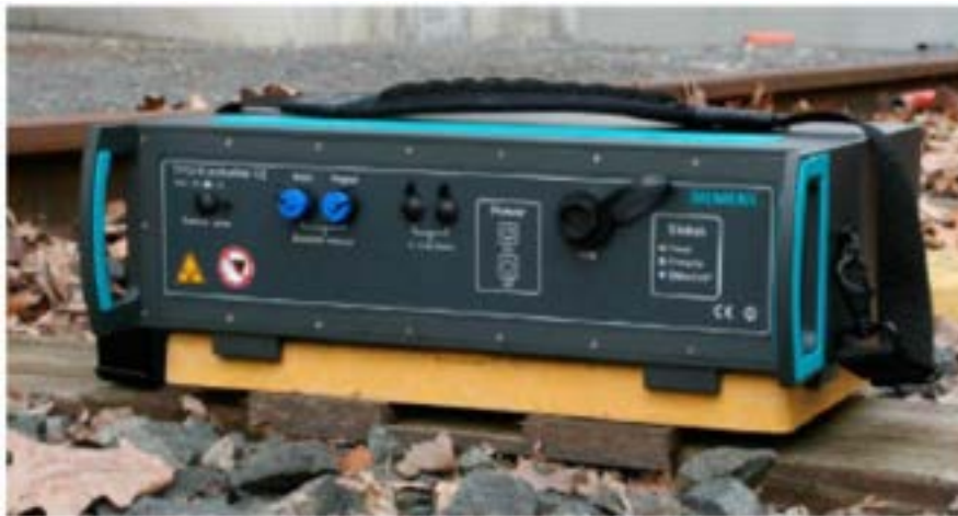
Figure 4 - TPG Base Unit Positioned on Eurobalise.
