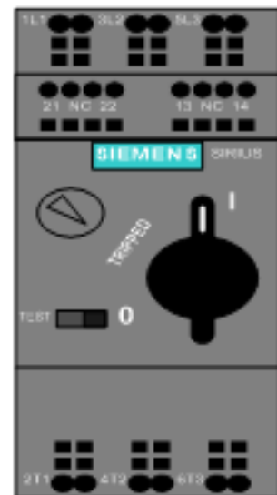
Figure 1 - Incoming supply switch
