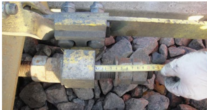
Figure 1 – Photo of Escapement Measurement
