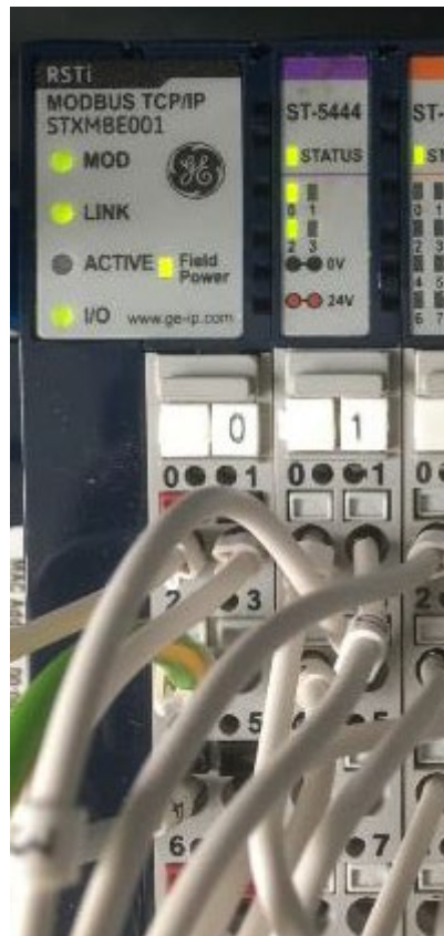
Figure 1 - RSTi ST Modules configurable fitted to a TCP-IP Network Adapter
