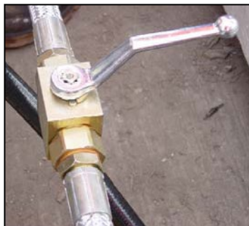
“Closed” Position (Normal Operation)
