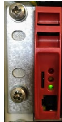
Figure 1 - Inverter Monitor Module
