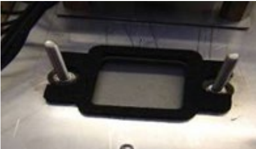
Figure 7 – New gasket fitted
