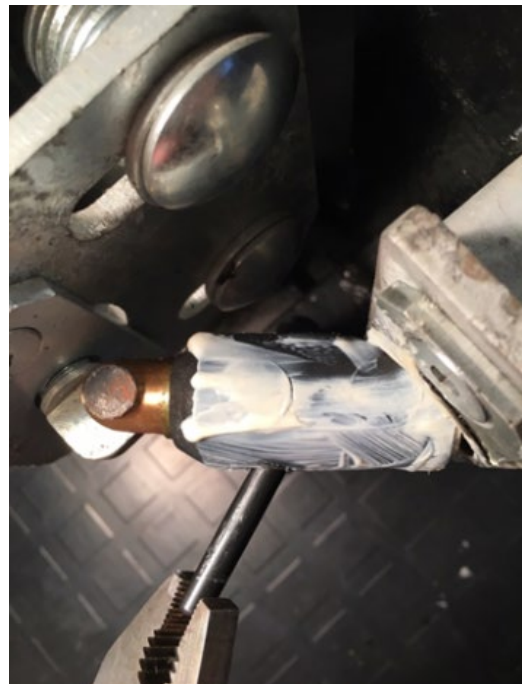
Figure 2 – Locking Pin Insertion
