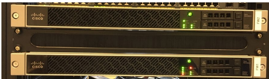
Figure 13 - Status Lights on Front of Firewall
