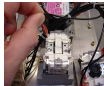
Figure 11 – Swapping Wiring to new contact block
