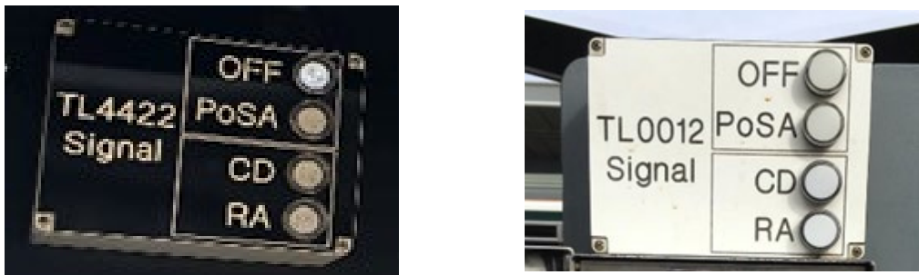
Figure 1 – Dispatch Interface Units
