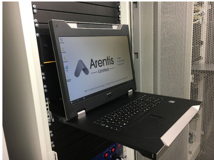
Figure 2 - KVM Monitor: Top view, extended position
