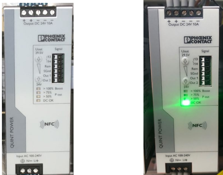
Figure 1 – QUINT PSU (Unpowered / Powered)
