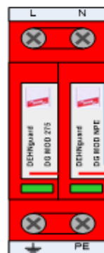
Figure 3 - Mains Supply Surge Arrestor
