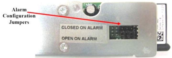
Figure 2 - Alarm Configuration Jumpers
