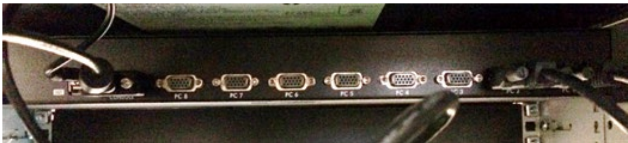
Figure 2 - Dell KVM Switch: Rear view
