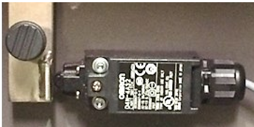
Figure 1 - Interlocking Safety Switch Brake Release
