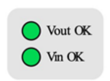
Figure 1 - PS module operational mode indications
