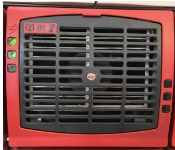
Figure 1 - GE UPS Inverter Module
