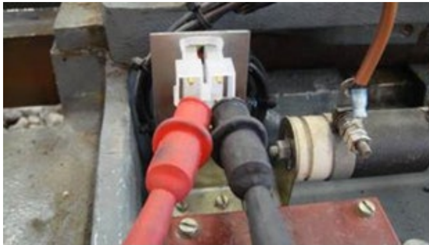
Figure 3 – Snubbing Circuit Resistance Testing Connections
