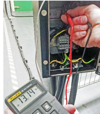
Figure 9 – Actuator Voltage Readings
