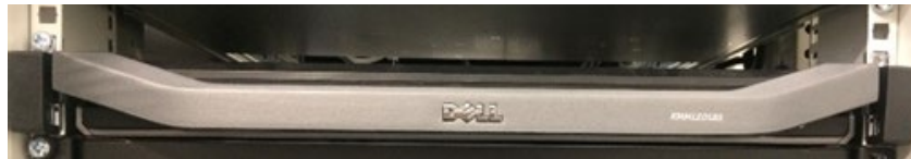
Figure 1 - KVM Monitor: Front view, stored position
