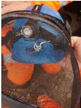
Photograph showing the piece of barbed wire embedded in the IP's mesh visor and the brush cutter.
