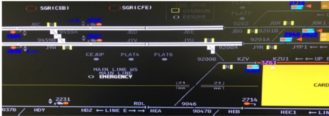
View of Cardiff Panel recreated – the white lines show the EPRs applied
