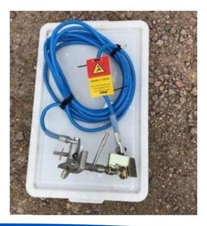
Following an isolation audit, it has become apparent that the industry is continuing to use the non-interlocked variant of long portable earths for earthing overhead line equipment.
