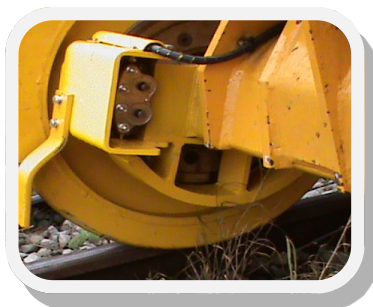
Picture 2 – Example of Type 9b RRV with knurled drive hub extensions
