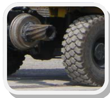
Picture 2 – Example of Type 9b RRV with knurled drive hub extensions
