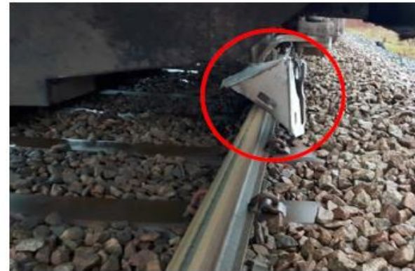
(Top right) FFC footage from train showing item on railhead (Bottom right) the signal wedge after impact, lodged in the wheel guard
