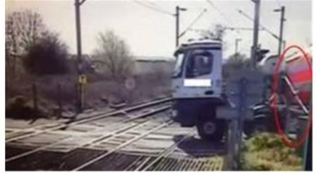
A further incident occurred on 2 May 2019 at West Bank Hall AHB level crossing in Yorkshire during road resurfacing. A tarmac lorry reversed onto the crossing and removed the downside barrier after the sequence started when a train approached. The freight train was able to stop just before the crossing.
