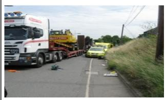
From marks at the scene, it is believed the front offside wheel mounted the kerb, onto a grass verge. It is believed the rear wheel failed to follow the front and was constrained by the kerb. It is believed the rear of the moving lorry crushed the injured person against his lorry.
