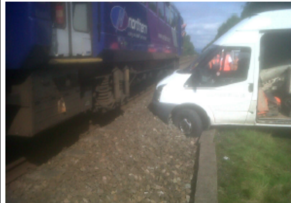
Vehicle within 1 metre of an operational line
