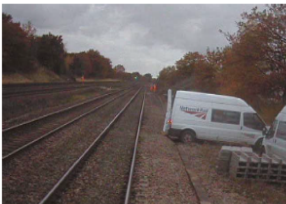
Vehicle door struck by passenger train
