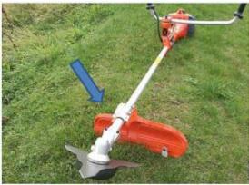
Protective guard fitted incorrectly
