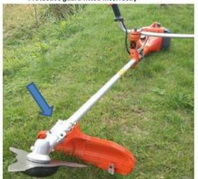
Protective guard fitted correctly
