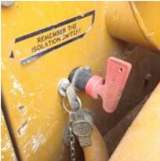
Isolator Key to be removed.
