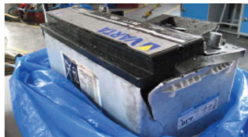
Damaged Varta Black Dynamic 590 122 072 battery. Issued by: Paul Conway Acting Professional Head (Plant and T&RS).
