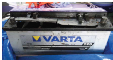
Damaged Varta Black Dynamic 590 122 072 battery. Issued by: Paul Conway Acting Professional Head (Plant and T&RS).
