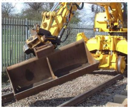
Most other attachments that could be fitted would require a machine controller to hold the appropriate attachment grouping or be a Crane Controller with the appropriate attachment group to control the "lift" as with any other lifting operation.
