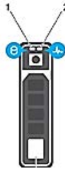
Figure 10 – LED locations on the Hard Drive
